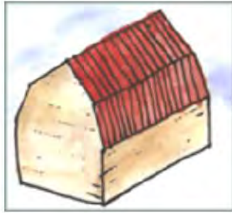
Gebroken dak (mansarde):
